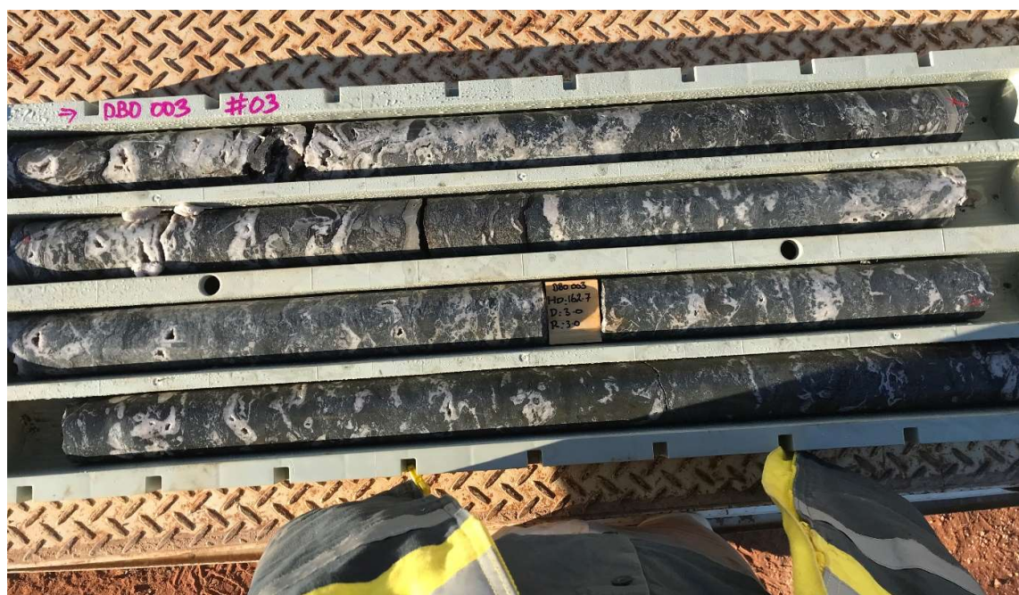
(Figure 5 - Wonawinta Deeps core from hole DBM003 showing carbonates hosting sulphides and high grade 5 Zn-Pb-Ag mineralisation as announced on ASX 8 February 2021)
