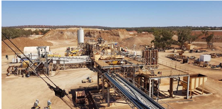
(Figure 8 - Wonawinta plant showing gravity circuit, regrind mill and ROM stockpiles in background)
