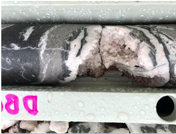
Figure 4: Typical sulphide mineralisation (galena and sphalerite) examples; along margins of quartz-filled vugs (top right, lower left); associated with brecciated quartz veins (top right); and in stylolites and interstitial matrix of fossiliferous dolostone (lower right). For scale, core widths are 64 mm (HQ)
