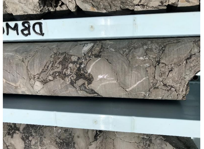
Figure 4: Typical sulphide mineralisation (galena and sphalerite) examples; along margins of quartz-filled vugs (top right, lower left); associated with brecciated quartz veins (top right); and in stylolites and interstitial matrix of fossiliferous dolostone (lower right). For scale, core widths are 64 mm (HQ)
