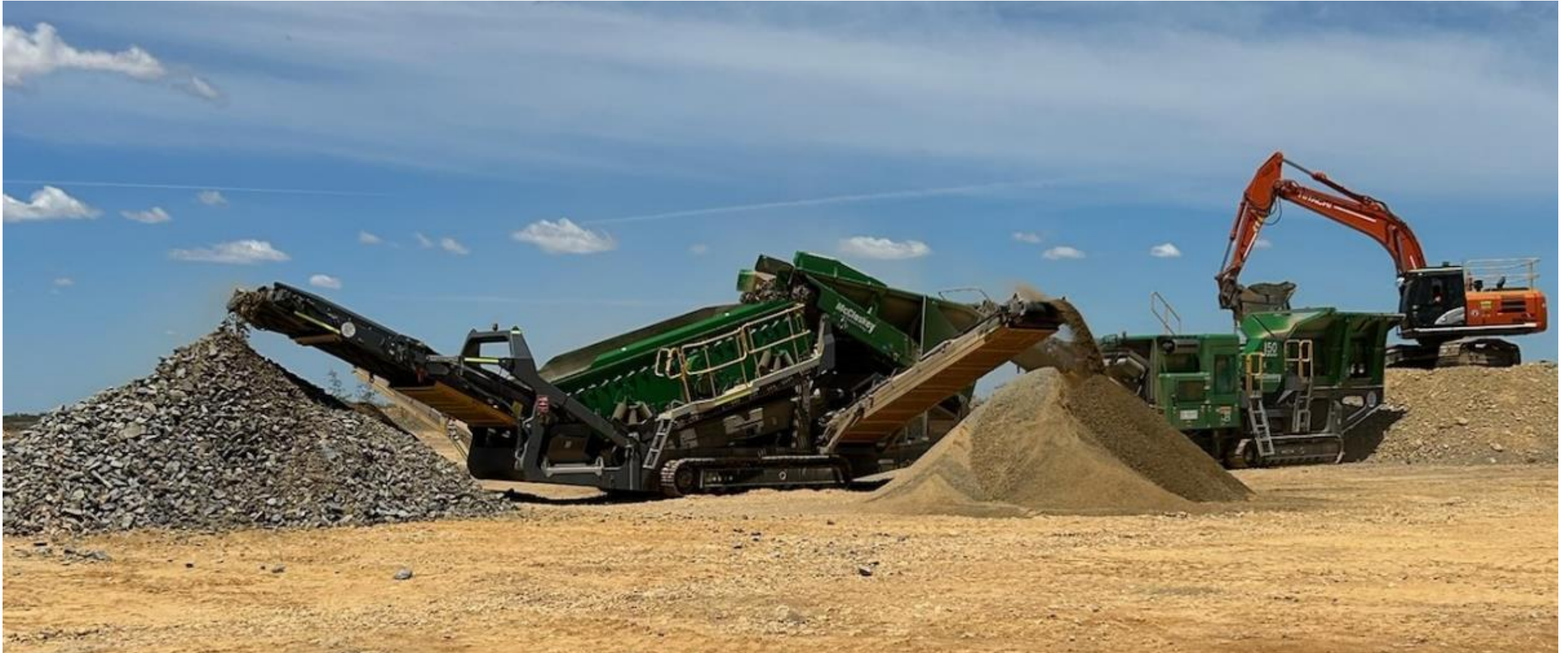
Photo of the McCoskey R230 'reclaimer' mobile screening plant at Mt Boppy.
