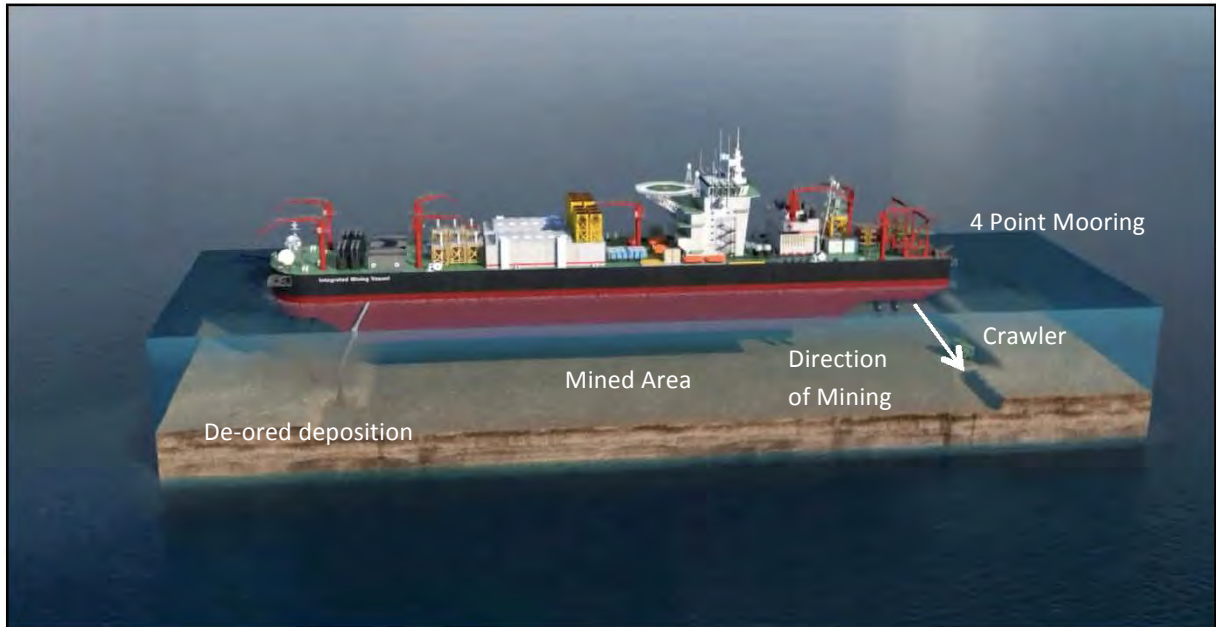
Figure 3: The Integrated Extraction and Processing Vessel.
