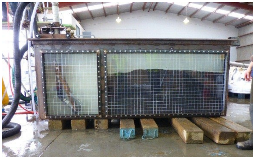
Figure 42 Breach Tank Used in Testing Seabed Sediment
