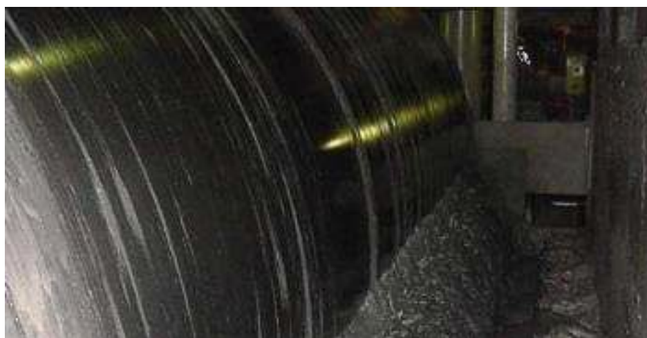
Figure 62 Magnetite Concentrate Exiting a Wet Drum Magnetic Separator
