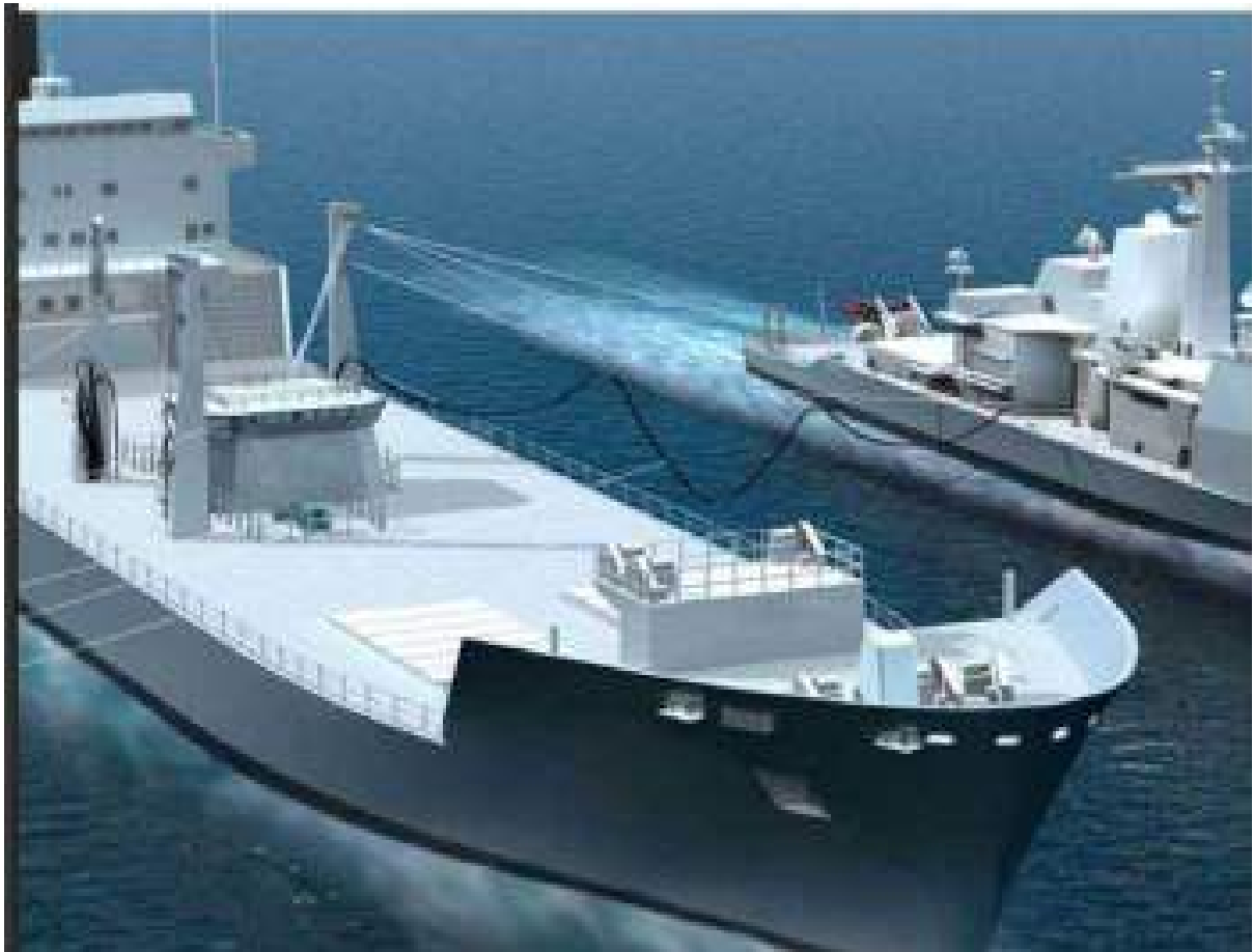
Figure 77 Typical Refueling Configuration
