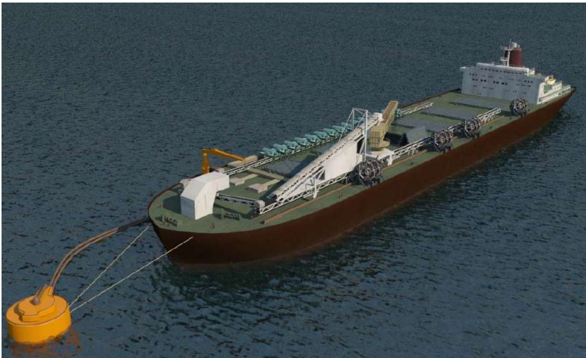
Figure 4: Illustration of a dewatering transshipper with gravity reclaim and loading boom
