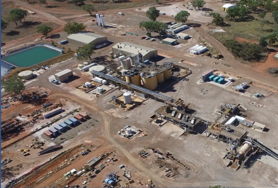
Figure 1 (left): Aerial view of the Existing Wonawinta 1Mtpa Processing Plant looking Southeast demonstrating the space available for potential future upgrades (e.g. addition of flotation cells to treat base metal ores). Figure 2 (right): Aerial view of the existing Manuka Open Pit looking south towards the existing Boundary Open Pit. A large portion of the Wonawinta silver deposit is free-dig and requires no drill and blast.
